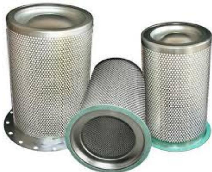
Air oil separators impress with efficient oil separation in compressors and vacuum pumps. Within the compression process of oil-cooled compressors, oil is used to seal, lubricate, and cool the air. Thanks to the coalescence effect, AOS reliably separate the residual oil contained in the compressed air, within the pressure vessel or a spin-on separator outside of the pressure vessel. The cleaned air is then available for the compressed air network.
